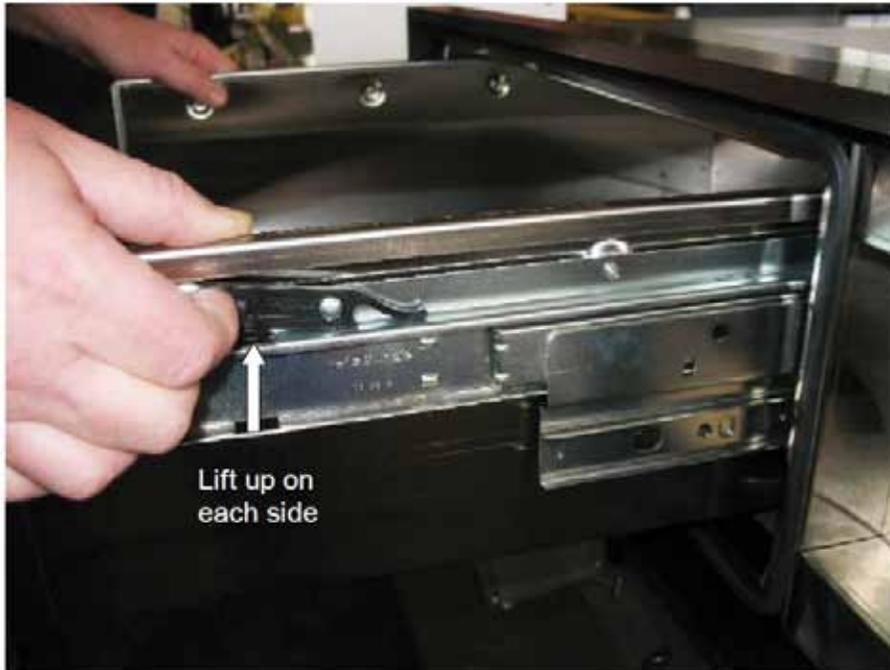
FIG 8 shows the drawer being lifted away from the drawer tracks. Remove and place on a protected surface.
