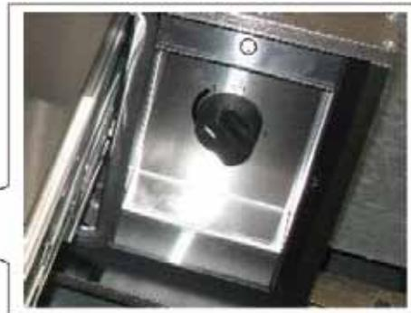
The temperature range of the warming drawer is between 90° F (Min) to 250 "F (Max) The temperature is control by the thermostat. In order to gain access to the thermostat and power connections, remove the unit from the cabinet to expose the right side access panel. FIG 3 shows the cover installed (Outlined with dotted red line)
