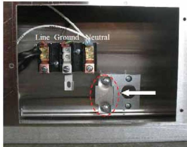
FIG 6 shows the Component compartment where the thermostat control is housed. The Capillary tube of the thermostat is routed through the side wall to the sensor. In this same location is where the heating element connections are located. One side is wired directly to Neutral. The other to the Thermostat. The indicator lamp is directly above the thermostat (Not shown)
